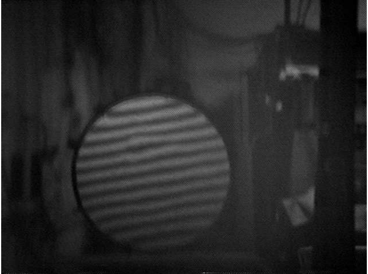
Figure 3: Ronchigram of the Dichromatic Cerenkov Mirror
