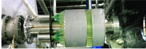
Figura 19: Intermediate-Ring Calorimeter.
