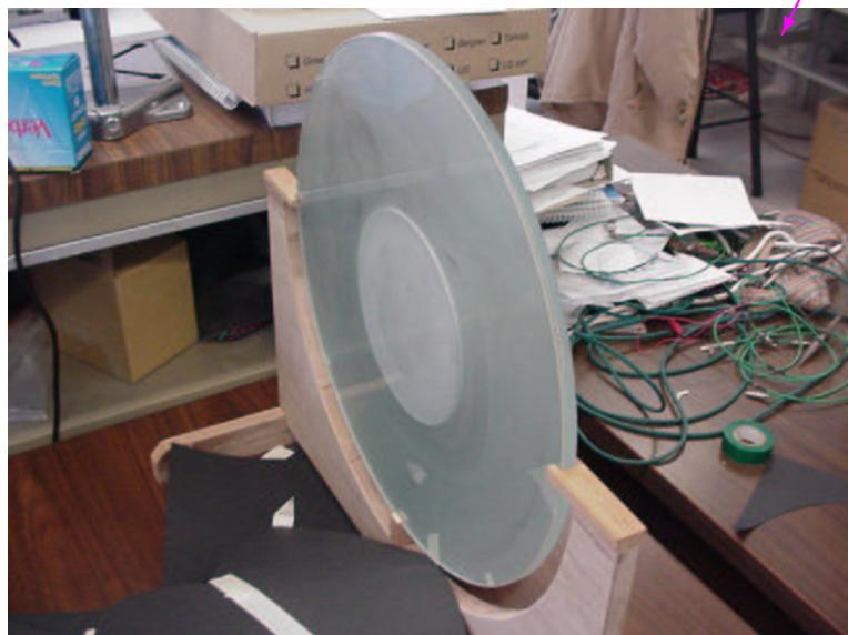
“Good” spherical mirror to test flat mirrors
