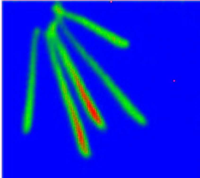
$\alpha$  particles in  $\text{CF}_4$  based gas mixture, recorded via scintillation in double-gem micro-strip gas chamber
