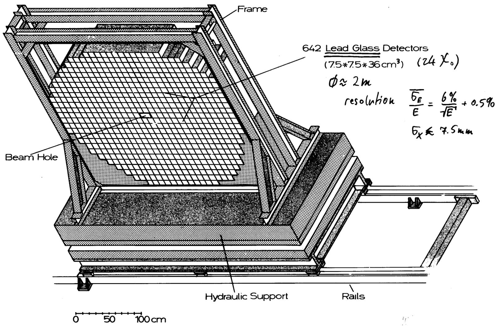
Lead-glass: Cherenkov light. Each block has one Photomultiplier attached.
